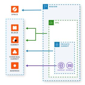
SOLIDserver IPAM has a very clever way to present IP network information to the network administrator. The object hierarchy is presented on nested views, from the entire VLSM topology down to the single IP address associated with an endpoint.
